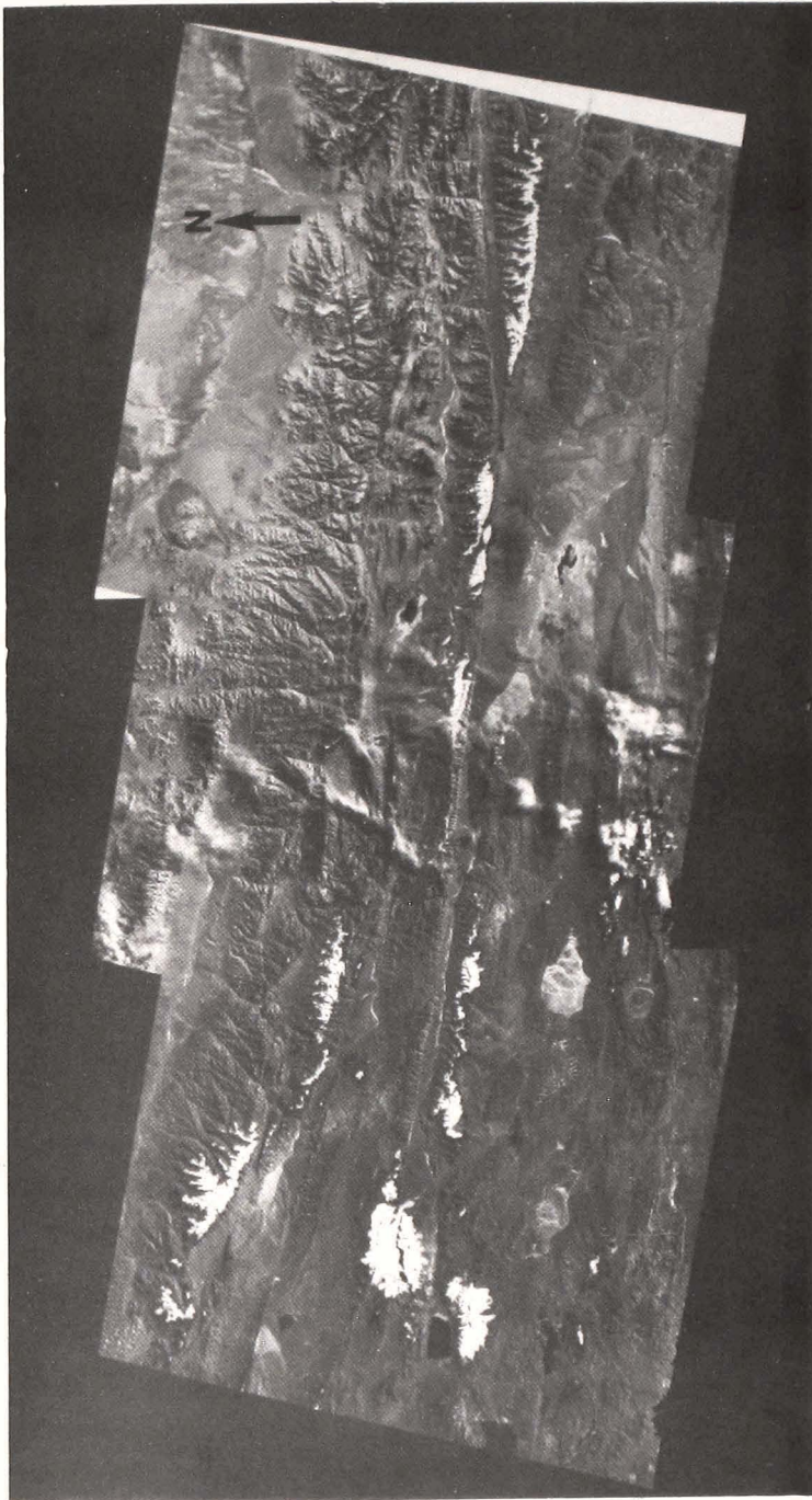
FIGURE 10. Mosaic of three Landsat images covering a portion of the western reaches of the Kunlun fault system. The main Xidatan-Tuosuohu-Maqu fault extends from about 90.5^{\circ} E to 95^{\circ} E on this mosaic. The traverse line crosses this fault in the Xidatan, near Kunlun Pass (see figure 9 to locate the mosaic). The minor faults and linear features identified in the area of the mosaic are indicated on figure 9. Locations of possible offset continuations of the phyllonite unit identified on these images are shown on figure 11.
